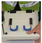
3 Use a Phillips Head Screwdriver to remove the four screws that secure the housing. Place the screws and washers in a safe place (such as small container or jar) to prevent loss. Hold the unit firmly and turn it over, face upwards on its base.
