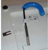
6 Unpack the replacement hook and lay in position over the plastic bracket.
