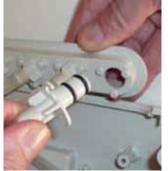
**6** Gently loosen the Connector Plate from the side of the unit and hold firmly in one hand.
