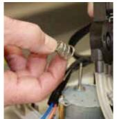
**9** Remove the spring and place it in a safe place for future replacement.
