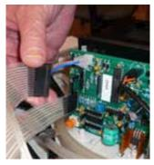
**11** Reconnect all seven leads into the corresponding connectors on the circuit board.
