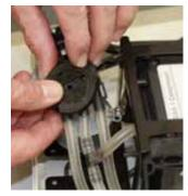
14 To test correct alignment of the motor and bracket, insert both bolts to secure the motor but finger tighten only. Gently place the rotovalve over the shaft to check the 'L' shaped bracket is correctly positioned to slide through the plastic handle at the side of the rotovalve. Once alignment is verified, remove the rotovalve and using the 7/32 inch socket wrench, tighten both bolts to firmly secure the motor in place. Be careful not to overtighten.
