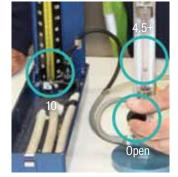
a Ensure the equipment is set to 'free flow mode' (i.e. no resistance or back pressure against the full flow of air from the compressor). The valve at the front of the Air Flow Meter should be fully open. If not, turn clockwise to open the valve to maximum. With the system in free flow mode, the ball bearing inside the Air Flow Meter should rise to a minimum of 4.5+ litres per minute. The Sphygmomanometer pressure reading should be low (approximately 10 mmHg).
