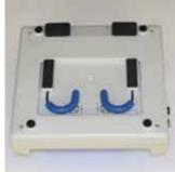
2 Using a soft cloth to protect the unit from damage, place the Control Unit on a level work surface with base facing upwards.
