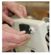
7 Unpack the replacement rubber feet. Insert the long nose of the rubber foot into the empty socket on the base of the unit (pushing from outside in).
