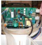
6 Disconnect the remaining three connections from the PCB (two flat digital leads and one air tube). Be sure to note the location of all seven connections on the circuit board for easy replacement.
