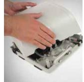
**10** Align the top and bottom housing before slowly pushing closed. Ensure the seal is properly aligned around the housing, including the air hose connectors, fuses and power connector.
