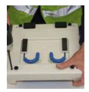
3 Use a Phillips Head Screwdriver to remove the four screws that secure the housing. Place the screws and washers in a safe place (such as small container or jar) to prevent loss. Hold the unit firmly and turn it over, face upwards on its base.
