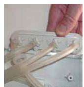
7 Remove the damaged connector from the Connector Plate by holding the base of the connector (at top of air hose) and twisting counter clockwise to release the locking mechanism.
