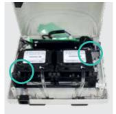
9 Before closing the housing, make sure all power leads and hoses are free from the side edges.
