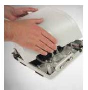
**11** Align the top and bottom housing before slowly pushing closed. Ensure the seal is properly aligned around the housing, including the air hose connectors, fuses and power connector.
