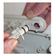
7 Detach all four connectors from the Connector Plate by holding the base of each connector (at top of air hose) and twisting counter clockwise to release the locking mechanism. Be careful to maintain the correct order of the hoses. You may want to gently secure hoses in the correct order using a gentle adhesive tape or cable tie to bind.
