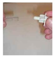
8 Detach the air hose from the damaged connector by pulling firmly. Unpack the replacement connector and press firmly to reattach the internal air hose as before. Ensure the hose is secure and fully buttressed against the base of the connector.
