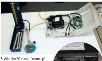
After the softmitte want up period has elapsed, detach the internal air hose from the compressor (some force may be required) and replace with the air hose from the Pressure Test Equipment (for directly connection to the compressor). Push the air hose firmly until it fully covers the connector.
