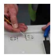
**3** Using a suitable tool (such as 2mm flat head screwdriver), gently press the clip on each air filter cover to remove.
