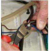
8 Using Wire Clippers (or a sharp knife) carefully cut and remove the cable tie securing the power leads between the two halves of the unit.
