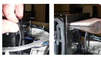
12 Secure the compressor to the metal cage by connecting the eight new rubber mounts, starting with four mounts on one side of the cage (bottom followed by top), then four mounts on opposite side.
