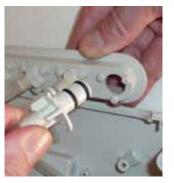
9 Refit the connector to the Connector Plate, twisting clockwise to lock into place. Repeat this process for other damaged connectors.
