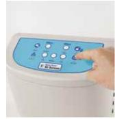
20 Connect the Control Unit to mains power and switch on the Control Unit to confirm operation.
