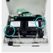
20 Before closing the housing, make sure all power leads and hoses are free from the side edges. Ensure the regulator tubing will not kink when the top cover is closed.
