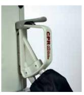
2 Check the Handle is securely attached to the Control Unit - all four connectors should be firmly inserted.
